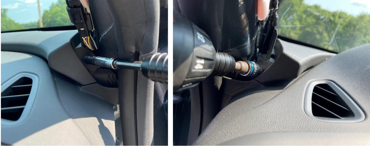
Now you are looking at three speakers held in by two screws apiece to unscrew. Remove, unplug, and set each speaker aside carefully.
