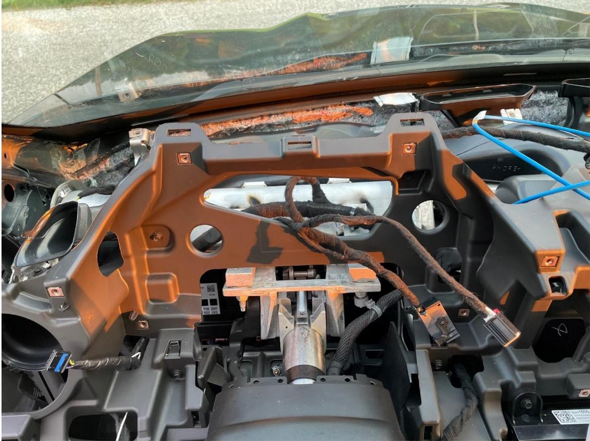
Remove the 2x 7mm bolts on the vertical plastic. Tight squeeze - pull on it to get the HUD in there.
