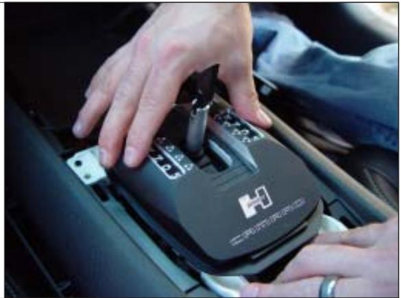
**STEP 21.** Replace the four (4) mounting screws.
