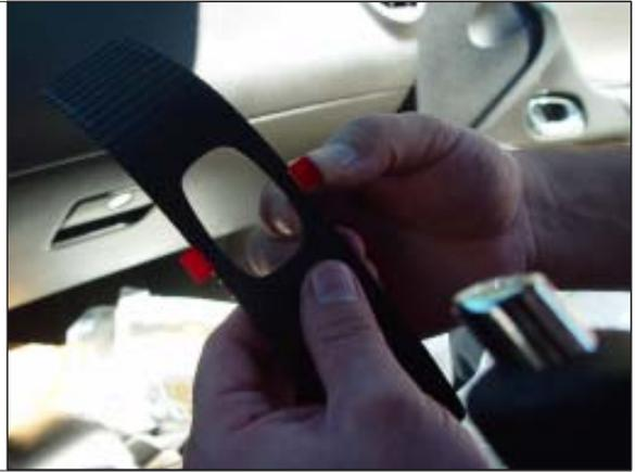
**STEP 13.** With the red indicator firmly in place. Apply a drop of instant adhesive into the back square access hole of the black plastic slider to lock the red indicator in place.
