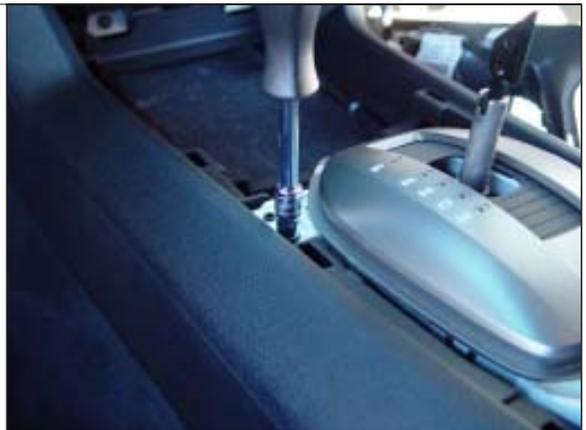
**STEP 8.** Unsnap the forward sections (both sides) of the center console side trim pieces.
