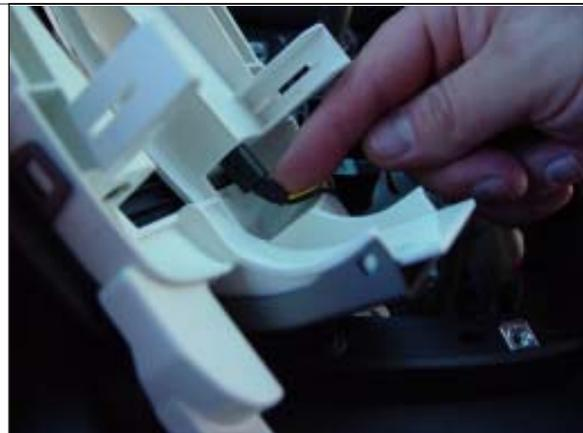
**STEP 11.** Carefully, unsnap the tabs of the shifter cover plate to remove it from the white plastic shifter frame.
