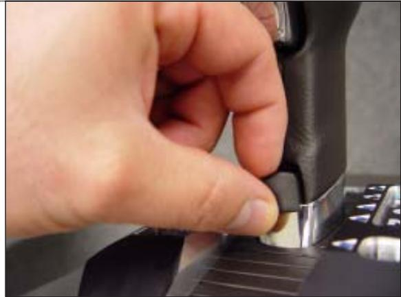
**STEP 26.** With the key in the ignition (vehicle "OFF") and foot firmly depressing the brake pedal. Cycle the shifter through all position to ensure smooth and accurate movement. If binding or rough movement occurs, review and ensure that all assembly steps have been completed as indicated.
