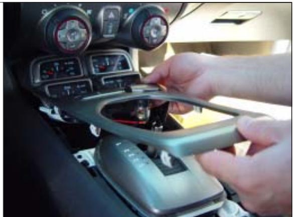
**STEP 7.** Unscrew the four (4) bolts holding the white plastic shifter cover frame to the center console.
