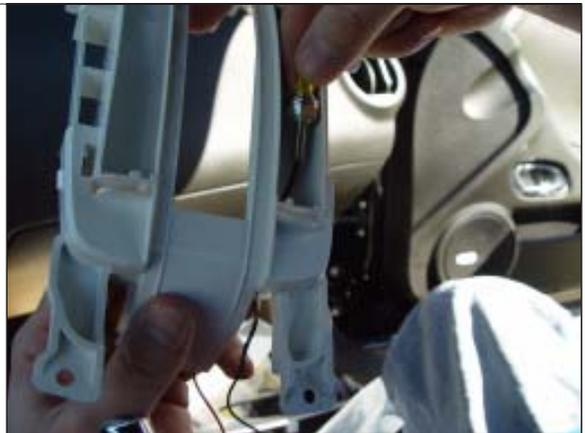
**STEP 15.** Ensure that the original LED bulb is NOT lit prior to beginning the wiring installation. This may require moving the shift lever to the park position and removing the key from the ignition. In some instances it may be necessary/prudent to disconnect the vehicle battery (refer to the vehicles service/owner's manual) to avoid problems with improper wiring.
