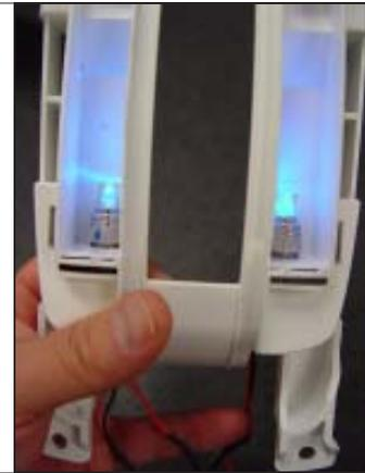
**STEP 19.** Place the black plastic slider into the track of the white plastic frame with the original red indicator on the driver's side of the vehicle (the newly installed indicator on the passenger side). Then snap the Hurst plate onto the white plastic frame making sure the cut-outs on the plate engage the tabs on the white plastic frame on all four (4) ears.
