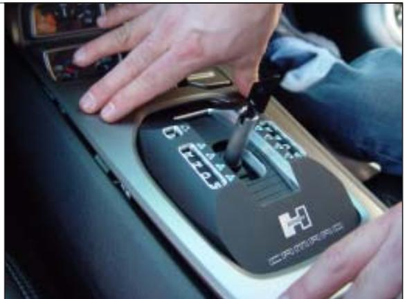
**STEP 24.** Reinstall the shifter knob by sliding it down onto the shifter shaft making sure that the base of the knob properly engages the black plastic slider. Then replace the mounting screw.
