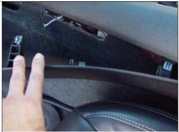
**STEP 23.** Carefully, replace the center console trim plate making sure that all mounting tabs snap into place.
