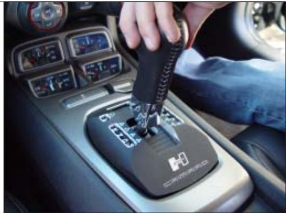
**STEP 25.** Reinstall the plastic access panel on the front of the shifter knob.
