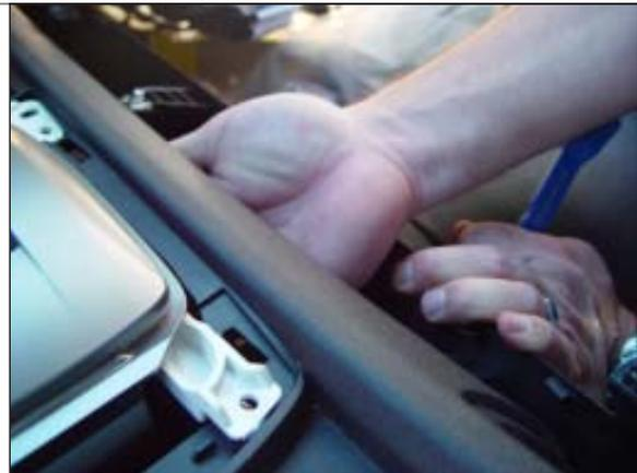
**STEP 10.** Lift the plastic white shifter frame and stock shifter cover out of the center console. Access the LED bulb and wiring and twist the bulb housing to disconnect it from the frame.
