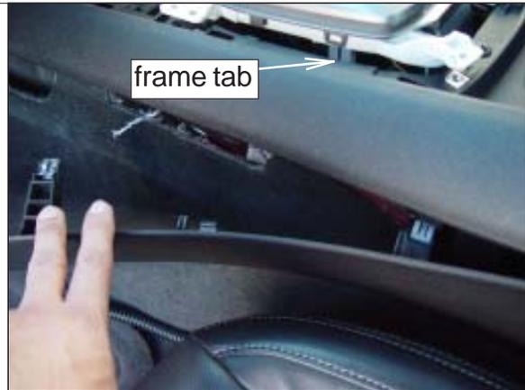
**STEP 9.** From under the center console access the white plastic shifter cover frame tabs on both sides and lightly pull the tabs outward to release the frame from the shifter assembly.
