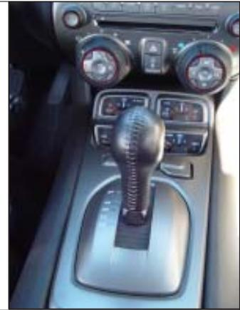
**STEP 2.** Carefully pry out the plastic access panel on the front of the shifter knob.
