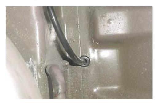
5. Route the tubing towards the back side of the plastic inner fender well.
