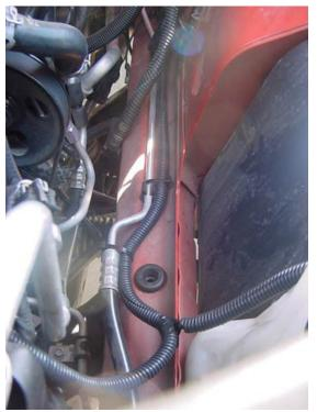
32. Route the second loom containing the tubing and the black wire (power wire for the horns solenoid) towards the left head light area to ensure it will not interfere with the reinstallation of the Air Box/CAI.
