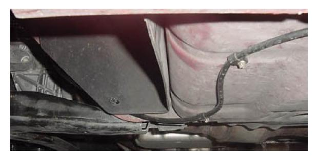
10. At this point, "thread" the tubing into the engine compartment, running it in between the frame rail and the steering linkage.
