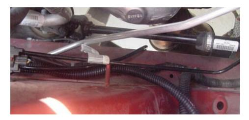
30. Using electrical tape, connect the two pieces of wire loom together and form a seal, such that they won't come apart. Also, wrap electrical tape around the loom at the point where the tubing entered the loom, such that it will not work itself out of the loom.
