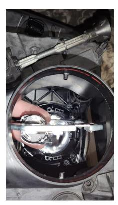
6. Remove the lens that is in the bottom of the housing. Turn it sideways, the same direction as the bracket to remove through the back of the housing.
