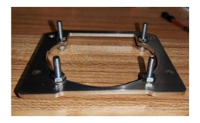
8. Install the bracket with the studs facing UP through the back hole. You will re-use the stock T20 screws to install the bracket. **Do not overtighten!** They are coarse thread into plastic. Take care as to not overtighten the screws as they will strip easily. Tighten just to a firm snug.
