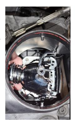
5. Remove the 4x T20 screws to release the bracket from the housing. Turn the bracket sideways with the solenoid side by the opening for the ballast (2nd Picture).
