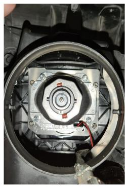
ballasts to your Morimoto D2S to D1S adaptor ignitor and install it in the 5 o'clock position (press it down onto the bulb) and rotate to the 6 o'clock position.
