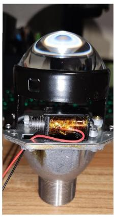
projector as shown to lower it in. You will need to ensure the wires are towards the bottom near the ballast opening as shown in the 2<sup>nd</sup> photo.
