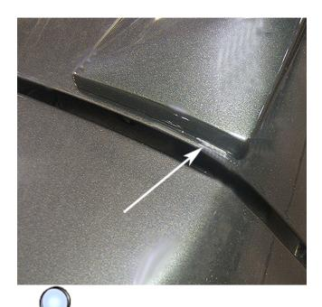
Some customers may comment that the rear compartment lid mounted spoiler is making contact with the rear compartment lid. This contact condition may cause paint damage to the rear compartment lid.
