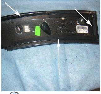
8. Install the two short and four long spacers on the underside of the spoiler in the same position as the original spacers.
