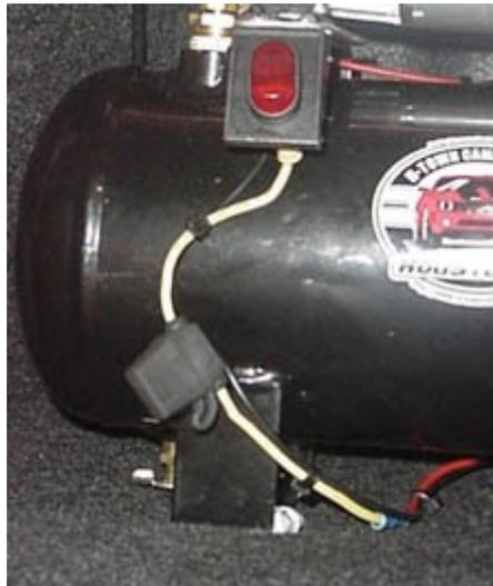
36. Connect the wire from the In-line Fuse holder to the POWER terminal on the rocker switch.
