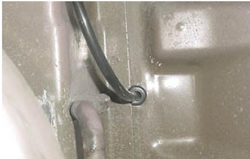
31. Run the tubing into the trunk. Ensure the end of the tubing has a straight clean cut. Place the tubing nut over the tubing. Install the ferrule onto the tubing, and install the insert into the tubing.
