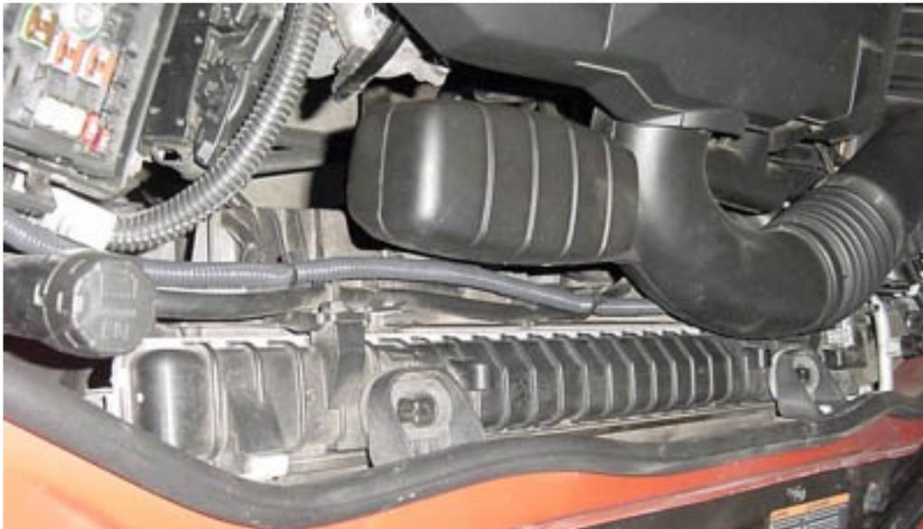
9. Insert the Black wire into the wire loom, starting at the fire wall end, stop where the loom will be at about the bottom of the radiator and leave the remainder outside of the loom at this time.
