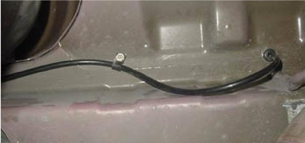
6. Route the tubing above the wheel well opening and behind the plastic inner fender well.
