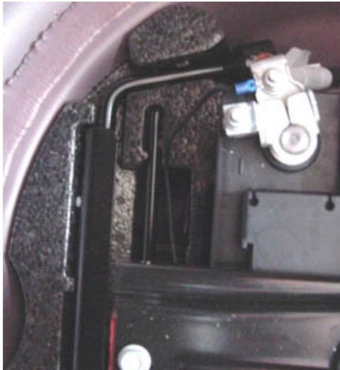
40. Connect the Red (power) wire to the post under the cap of the POSITIVE terminal post.
