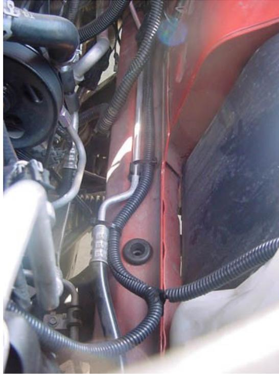
32. Route the second loom containing the tubing and the black wire (power wire for the horns solenoid) towards the left head light area to ensure it will not interfere with the reinstallation of the Air Box/CAI.
