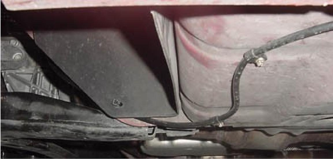
10. At this point, “thread” the tubing into the engine compartment, running it in between the frame rail and the steering linkage.
