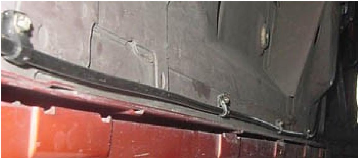
9. At the front of the car, route the tubing towards the inner fender well, and go under it and up and over the frame rail.
