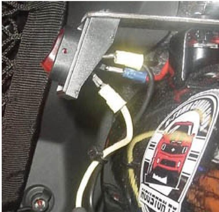
20. Take Red (Load) and Black (Ground) wires from the pressure switch and cut them to the proper length to reach the new rocker switch.
