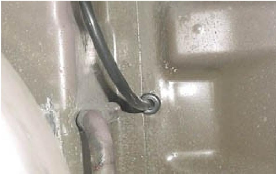
5. Route the tubing towards the back side of the plastic inner fender well.
