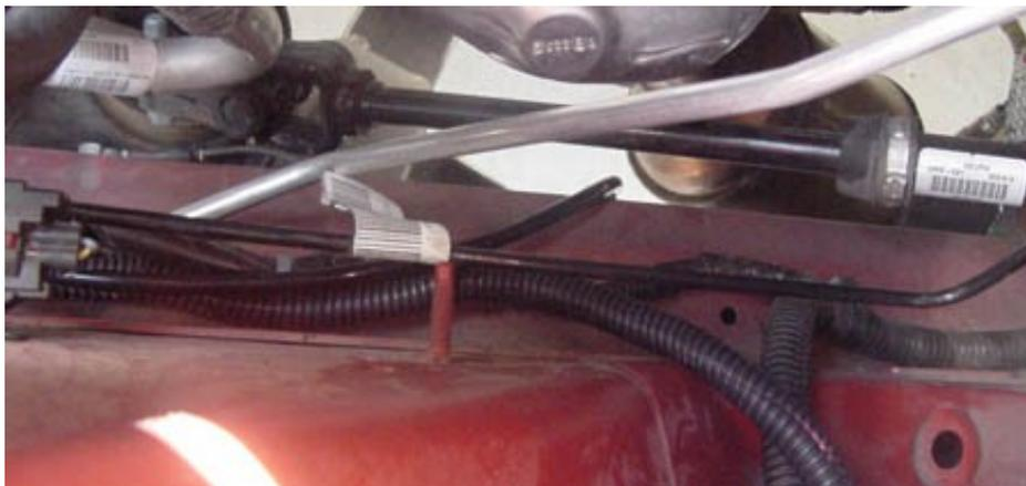
30. Using electrical tape, connect the two pieces of wire loom together and form a seal, such that they won't come apart. Also, wrap electrical tape around the loom at the point where the tubing entered the loom, such that it will not work itself out of the loom.
