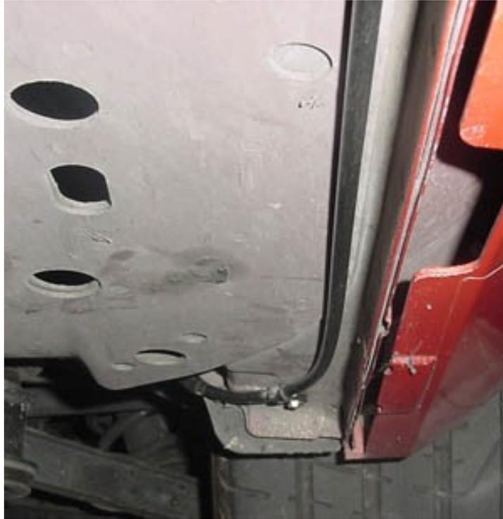
8. Continue on down the side drilling and installing tubing clips just inside the rocker panel, the full length of the car up to the front left wheel well.
