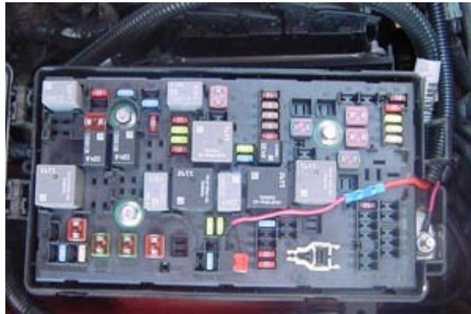
6. Attach a long piece of RED wire using a “splice crimp” or solder and shrink wrap if you prefer, which will be long enough to run from the fuse box, across the top of the radiator and down the side, to the top of the frame rail and to the firewall where it will penetrate, plus another 3 feet.
