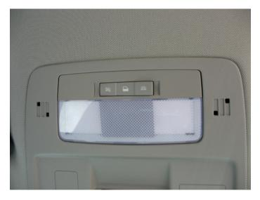
4. Test it with the light on. As you can see here, the yellowish bulb combined with the white cover makes this dark purple gel look pink (afternoon picture). You can also see some light leakage around the edges.
