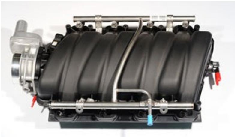
*The LS7 intake is a bit different than that used previously. Obvious is its rectangular rather than round ports. Maybe not so obvious is a bit less runner length to better suit the LS7's torque curve. Image: Author.*
