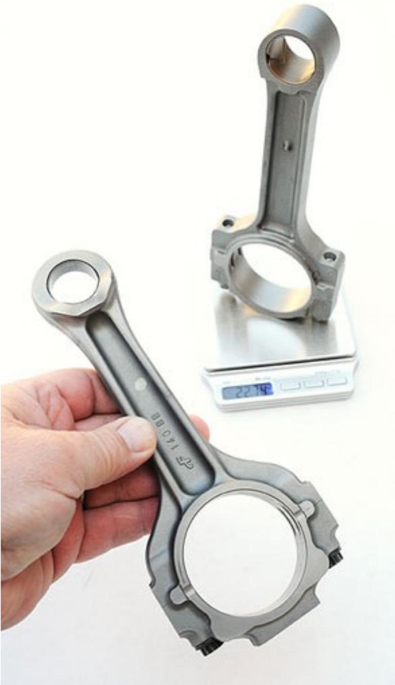
said. *"It was an investment-cast (steel) con rod. It had a lot of mass lightener pockets—less material (than a forged LS6 rod) to keep the mass down. However, with the seven-liter, the longer stroke and higher engine RPM was a concern for proper oil film thickness.*
