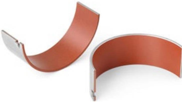
**An LS7 rod bearing with its obvious red, polymer coating. In a short period after the first engine start, some of the red wears away leaving the anti-friction polymer coating to fill the microscopic voids in the surface of the aluminum. Image: GM Powertrain.**
