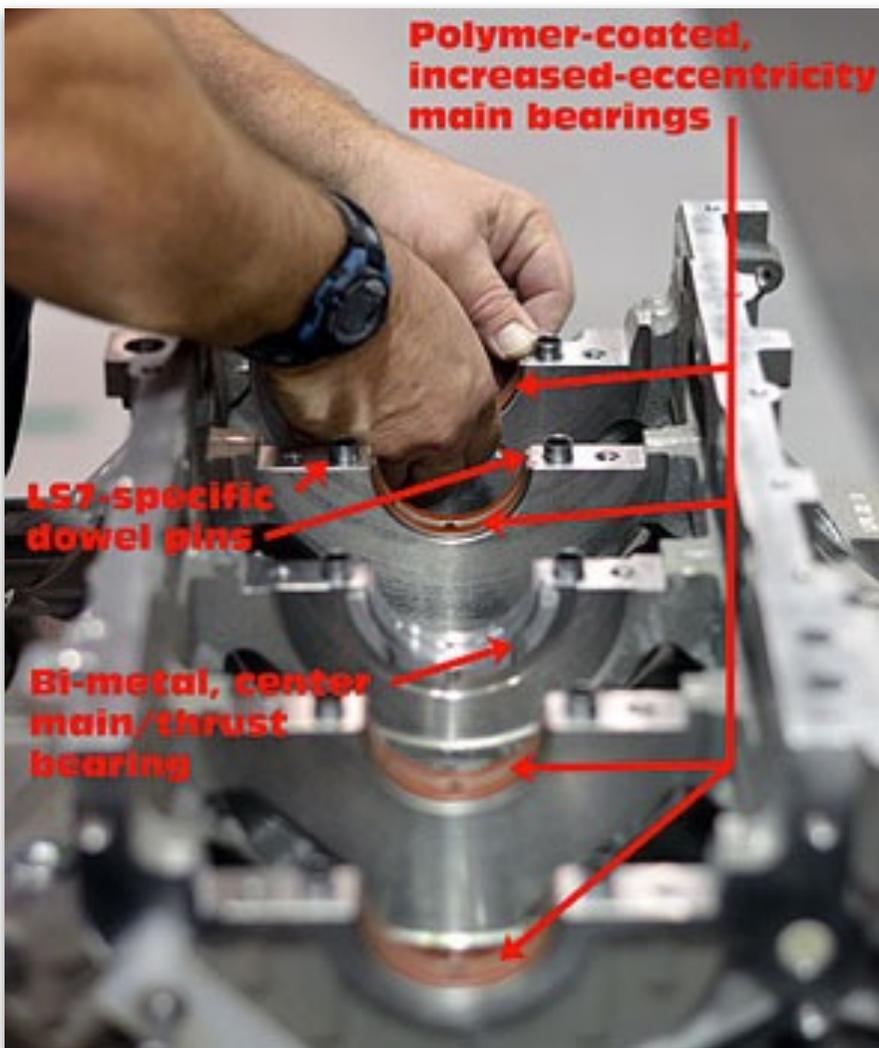
**LS7 main bearings being installed at the PBC. Mark Kelly/GM Powertrain.**
