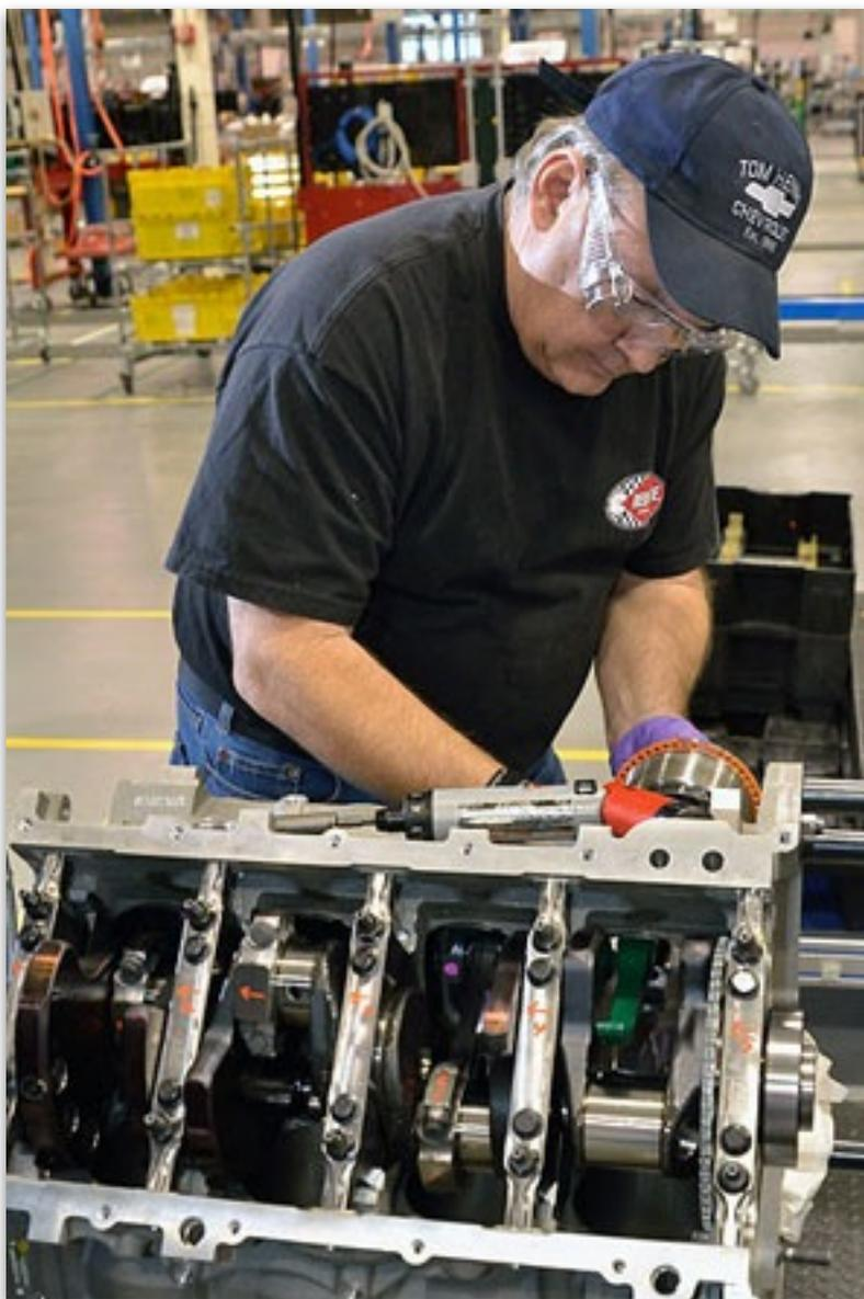
*During engine assembly, techniques similar to those used in the engine shops at Katech or Hendrick Motorsports are used to install the pistons, including an awesome ring compressor which the author insists would look excellent in his tool box. Image: Mark Kelly/GM Powertrain.*
