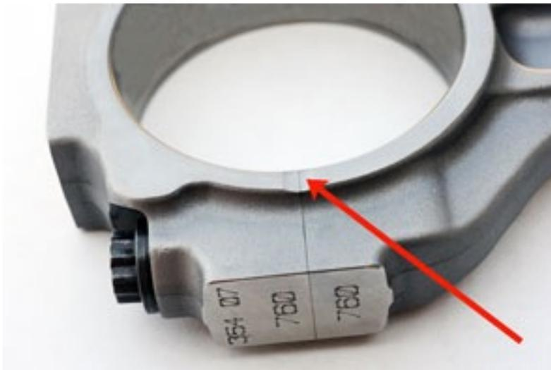
*The arrow points to the groove or divot which was added to LS7 rods to combat Ti dust. Image: Author.*
