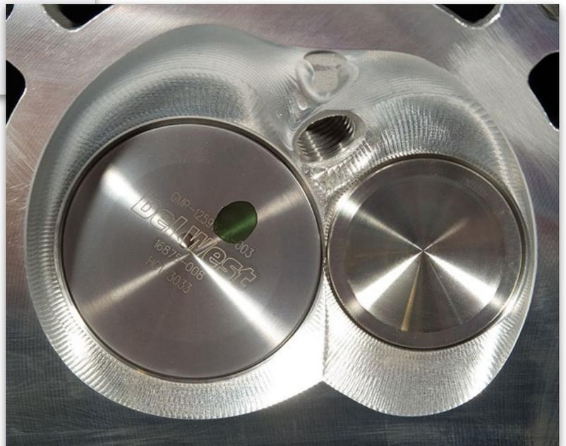
"We had to make a change and going to a thicker-head steel valve wasn't an option," Hicks continued, "because we wanted a 7000 RPM red line. We looked at a couple of alternatives—some really kind of radical. ultra-light steel valves. I tested a few of those and they failed miserably. Then we said, 'Alright. We gotta do what ever it takes.' We went to the titanium for
