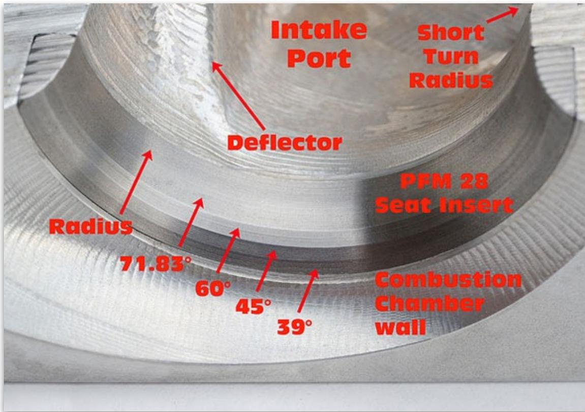
*This image details the space near the intake valve seat. The LS7 intake seat and transition areas are a very sophisticated system intended for one goal: maximum air flow. Image: Author.*
