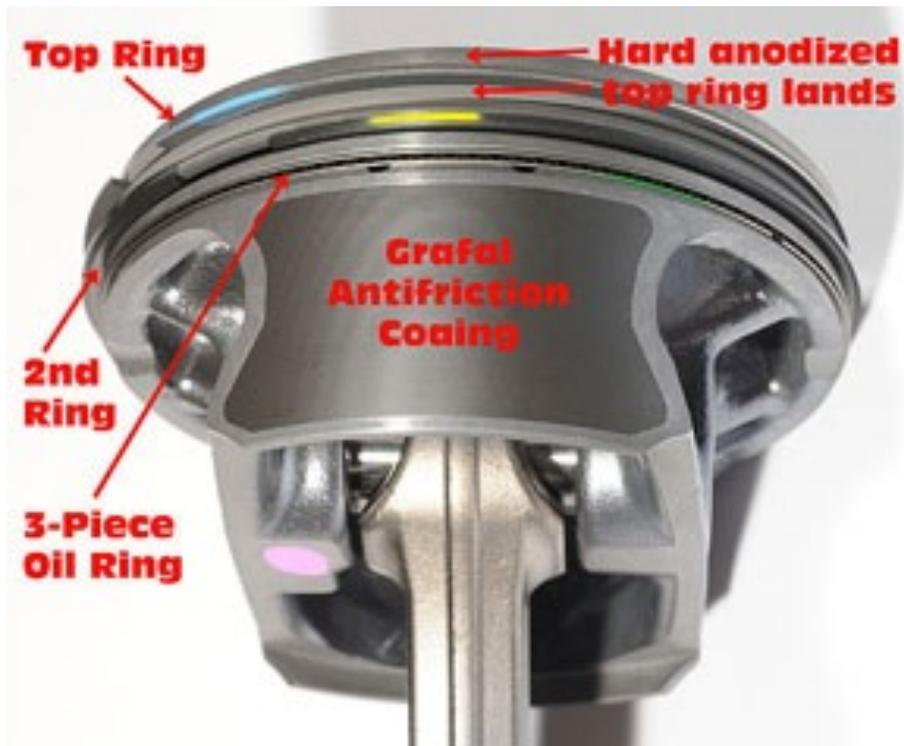
Areas immediately adjacent to the top ring groove are hard anodized and the surfaces of the piston skirts are coated with Grafal, a polymer-based antifriction material pioneered by Mahle with the 2002 LS6 piston.
