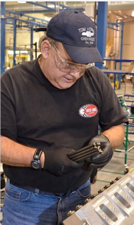
*LS7 pushrods are longer and have a thicker wall than do other Small-Block units. From a performance standpoint, the weight of the pushrod is not as important as it's stiffness. Image: Mark Kelly/GM Powertrain.*
