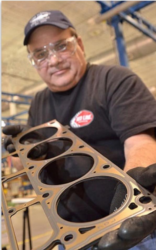
***The LS7 head gasket is standard fare for today's high-performance engines, a 3-layer, multilevel-steel (MLS) design.***
