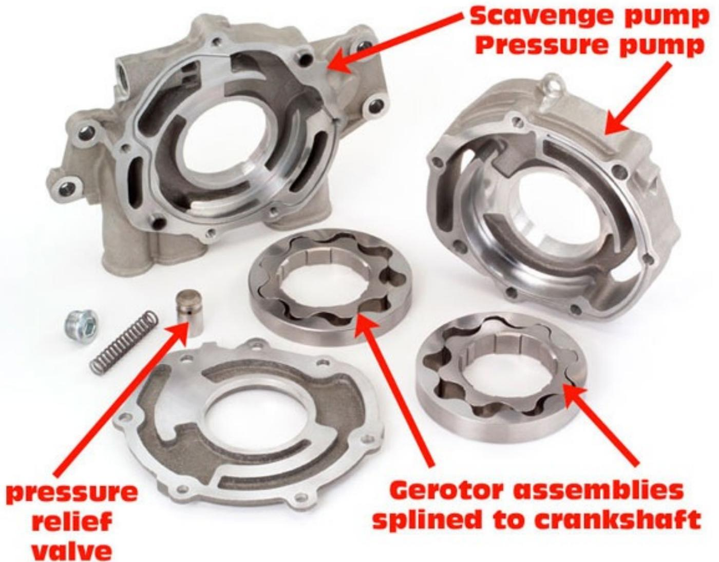
*LS7, two-stage oil pump components. Image: GM Powertrain.*
