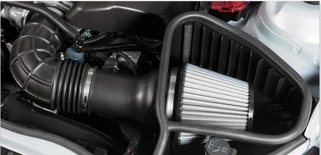
*Because of the limited space under a Camaro's hood, the LS7 air filter assembly and air duct had to be a unique design. Obviously, the 90° bend adds restriction compared to the C6 Vette design, so the Z/28 uses a conical, oil-cotton air filter element to gain back some of that lost airflow. Image: GM Powertrain.*
