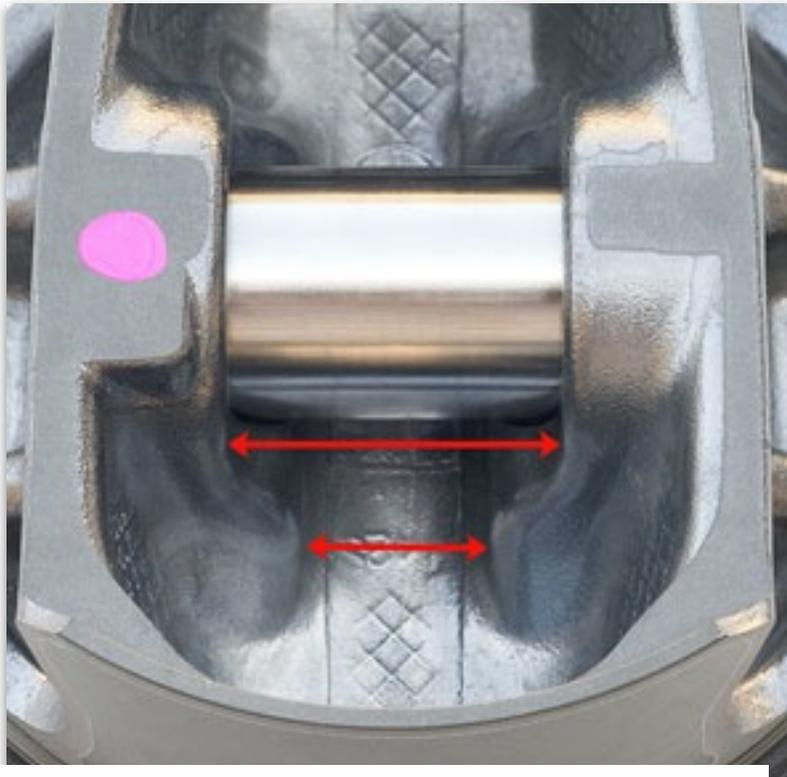
*Again, looking at the underside of the piston, to increase strength, the top portion of the wrist pin bore bosses, indicated by the shorter arrows, are wider than the bottom portion. Image: Author.*
