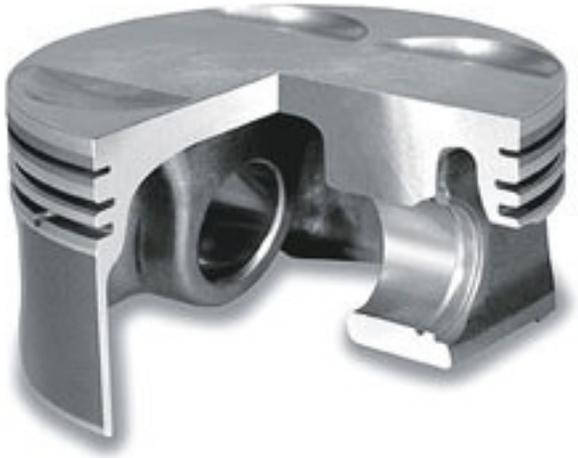
*This cutaway Mahle Ecoform piston, while not an LS7 unit, is typical of pistons made with that process. It is very light because of cavities the process forms in the underside of the piston which could not exist in a forging. Image: Mahle.*
