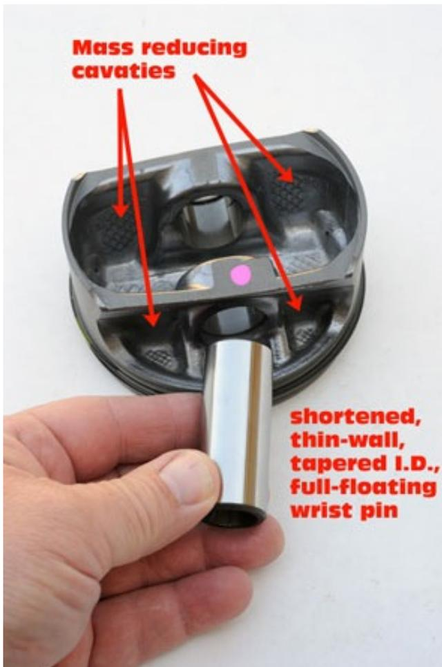
The LS7 piston has "asymmetric" skirts with the major thrust face being wider than the minor face, a configuration responsible for another slight mass decrease. The skirts are coated with "Grafal", Mahle's proprietary, polymer coating which reduces friction, increases scuffing resistance and allows less piston-to-bore clearance leading to less engine noise.
