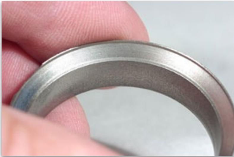
***A copper-infiltrated LS7 exhaust valve seat prior to installation in the head. Image: Author.***
