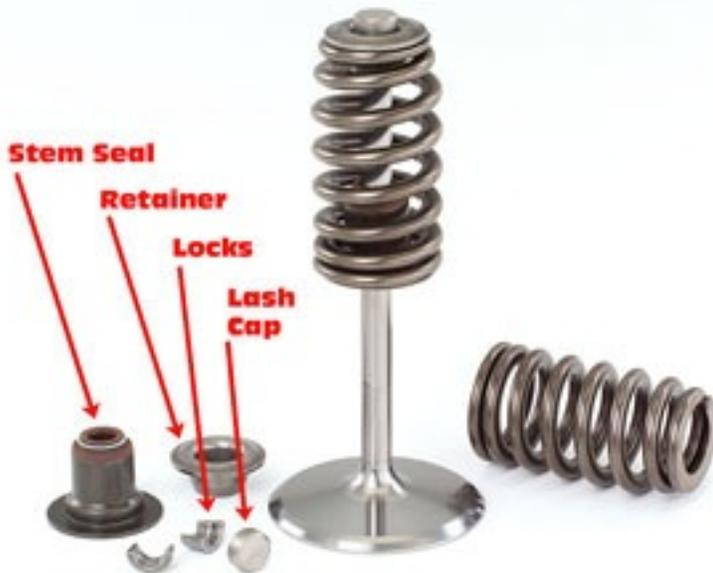
*Lash caps go over the tip of the stem of a titanium valve and prevent direct contact between the rocker arm and the stem. Without a lash cap, the stem of the Ti valve and the rocker arm tip would quickly wear. "Beehive" springs have been used on Gen 3/4/5 engines since the Camaro LS1 was introduced in 1998, however, the LS7 uses a specific beehive spring with more height and higher open pressure. Image: GM Powertrain.*
