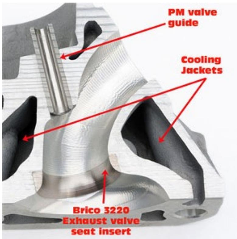
The exhaust port—the parts of the chamber just below it have the same type of turn radii and transition areas. You can see why LS7s exhaust ports flow really well. Image: Author.
