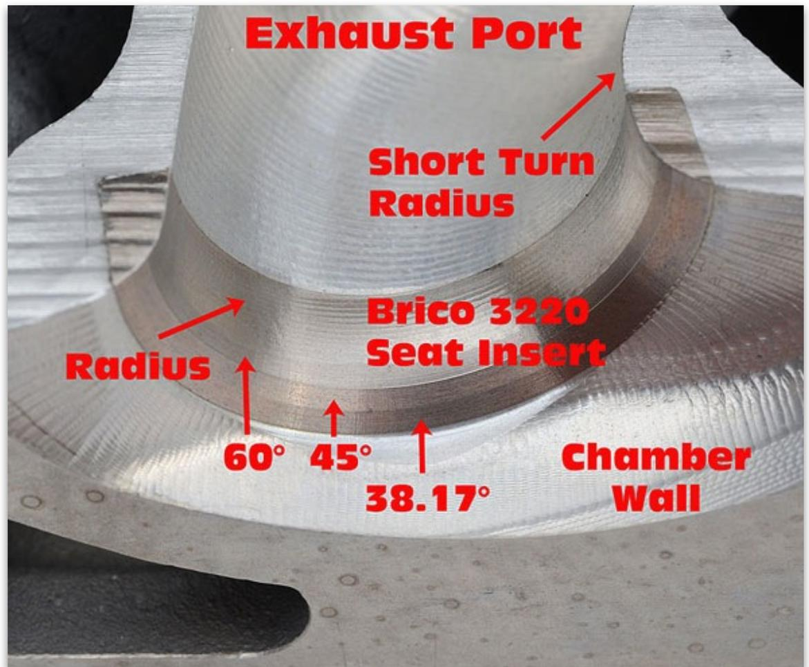
*The surfaces in the vicinity of the exhaust valve seat are designed with optimal exhaust gas flow in mind.*
