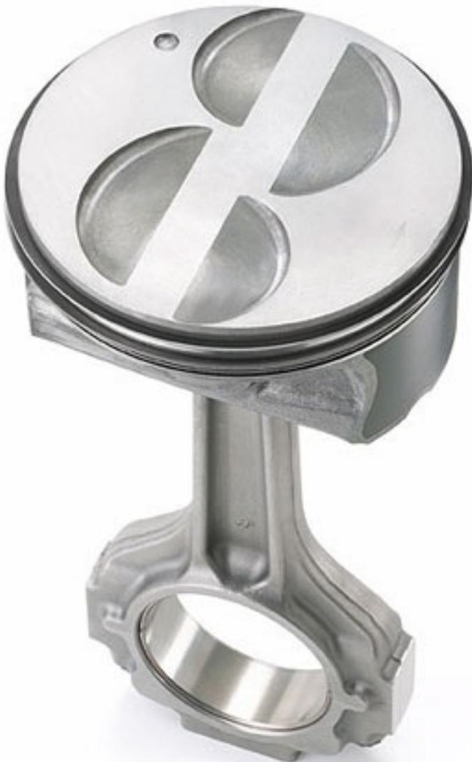
*An '06-'11 Corvette LS7 piston/rod assembly. The Camaro unit is identical except for a polymer-coated, bi-metal rod bearing. The four valve reliefs are a welcome feature of the piston top for those wanting to go to an aftermarket cam profile. Image: GM Powertrain.*
