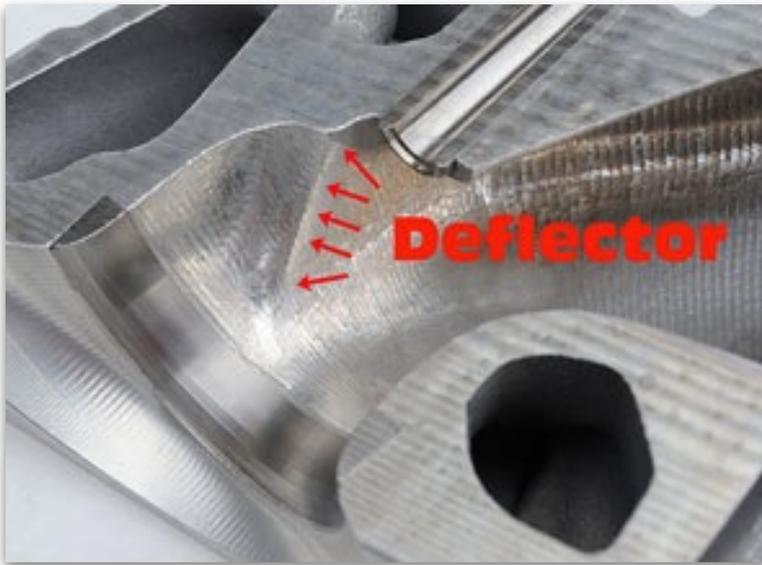
*The deflector which was added to the intake port just above the valve after research on Chapman Racing's wet flow bench. What's to bet half the head porters who've tried doing LS7 heads, grind that away? Image Author.*
