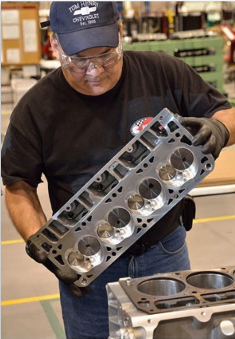
*The most important part on the engine is this cylinder head. Ti intake, raised ports, rolled-over 3° and fully CNC'ed. It's the key to the LS7's amazing performance. Image: Mark Kelly/GM Powertrain.*
