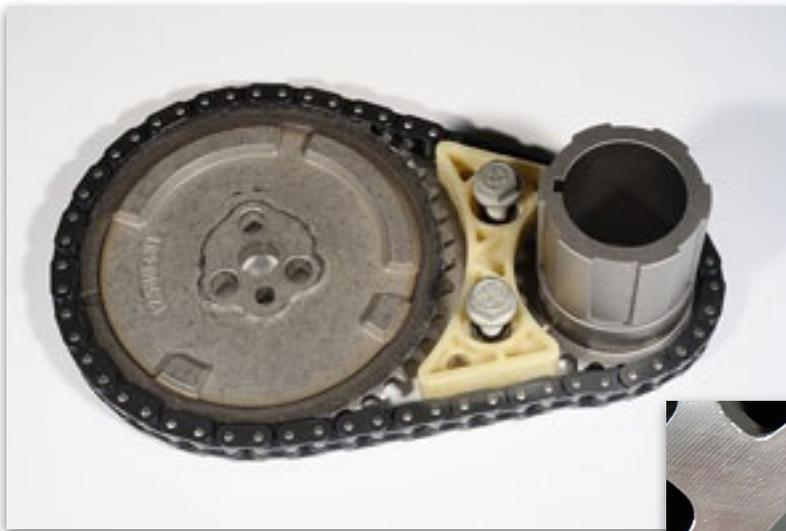
*Back in the day, people thought any high-RPM application needed a dual-row, timing chain, but in recent years, GM has developed some pretty stout single row, true rolling chains. Evidence of that is the LS7's timing set. Still not convinced? The Katech chain set, as used in the C5-R 427s, is, also, single row. Image: Author.*
