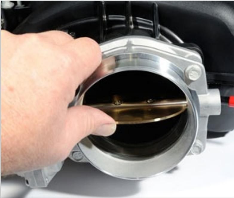
*The LS7 throttle bore is 90-mm, biggest in GM. Even the LSA's throttle body has only an 87-mm bore. Image: Author.*
