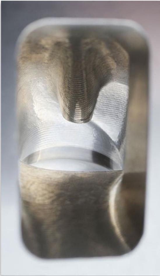
Near the end of the LS7 cylinder head development, Gerdeman and his team looked beyond just air flow. They studied how the air and fuel mixed in the chamber as it flowed across the valve seat and as it continued to mix once the intake valve closed and the compression stroke began. They, also, looked at the homogeneity of the mix near the spark plug and, once the ignition kernel developed, how the flame front propagated across the combustion chamber.
