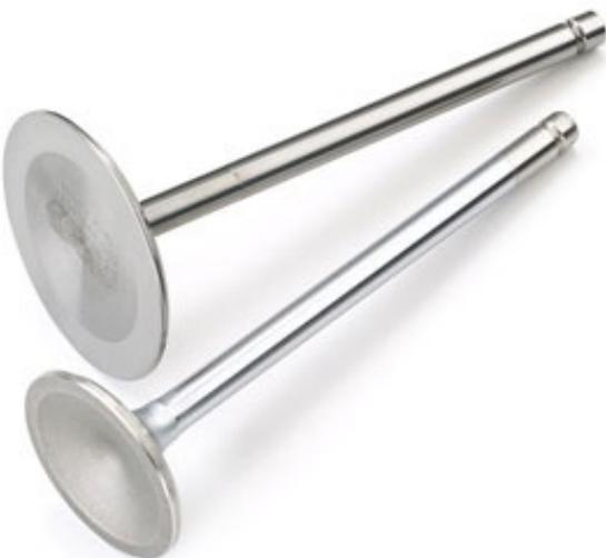
**Racy stuff—titanium intake and hollow stem exhaust valve. The stems are gun drilled, filled with sodium, the SilChrome head is welded in place, then the valve is machined.**
