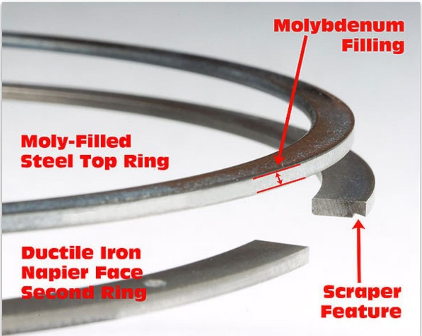
*The top ring is filled with moly as an antifriction measure. The LS7's Napier second ring was developed for the 2002 LS6 and later used on all Small-Blocks. A "Napier ring" has a distinct shape that enhances oil control by scraping oil off the cylinder walls as the piston moves down in the bore. Image: Author.*
