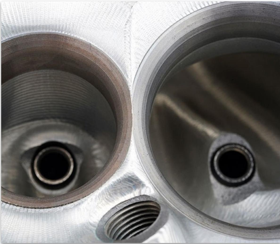
***A key development in the early stages of the LS7 head program was going to siamesed valve seats. That unshrouded the intake valve thereby improving airflow. Image: Author.***
