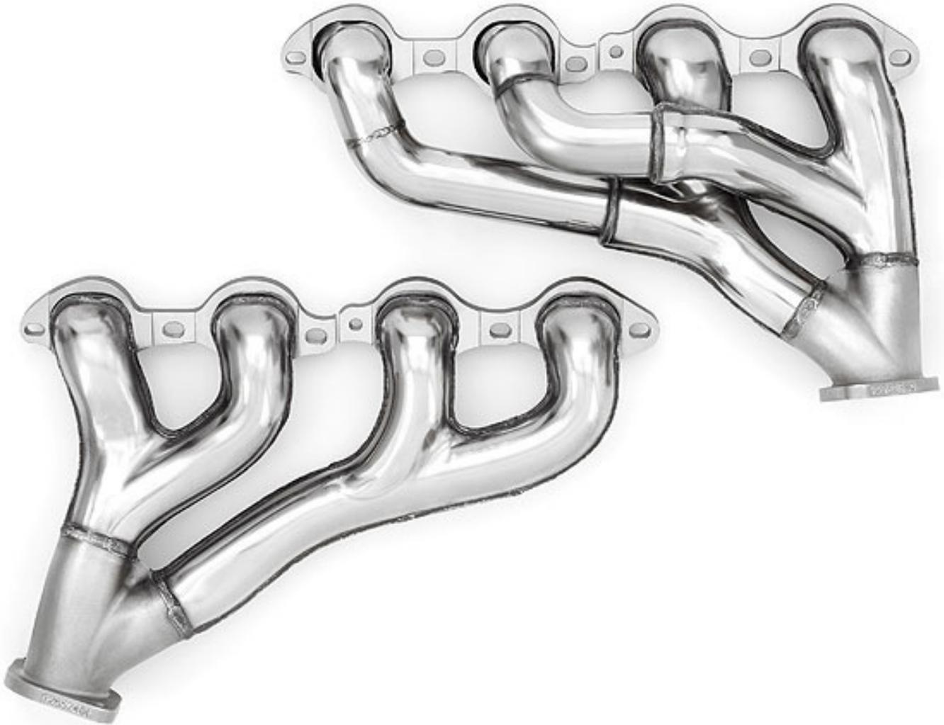
***The Camaro LS7 exhaust manifolds. Again, limited underhood space forced a somewhat more restrictive design than used on a Corvette so, GM went with a stainless steel, Tri-Y configuration which tucks in close to the engine and exits near the rear of the block, rather than the C6 Z06/ZR1 unit, which is a shorty header with a center exit. Image: GM Powertrain.***
