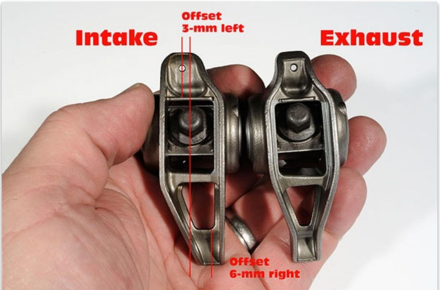
*A pair of LS7 rockers showing the offsets of the intake part.*
