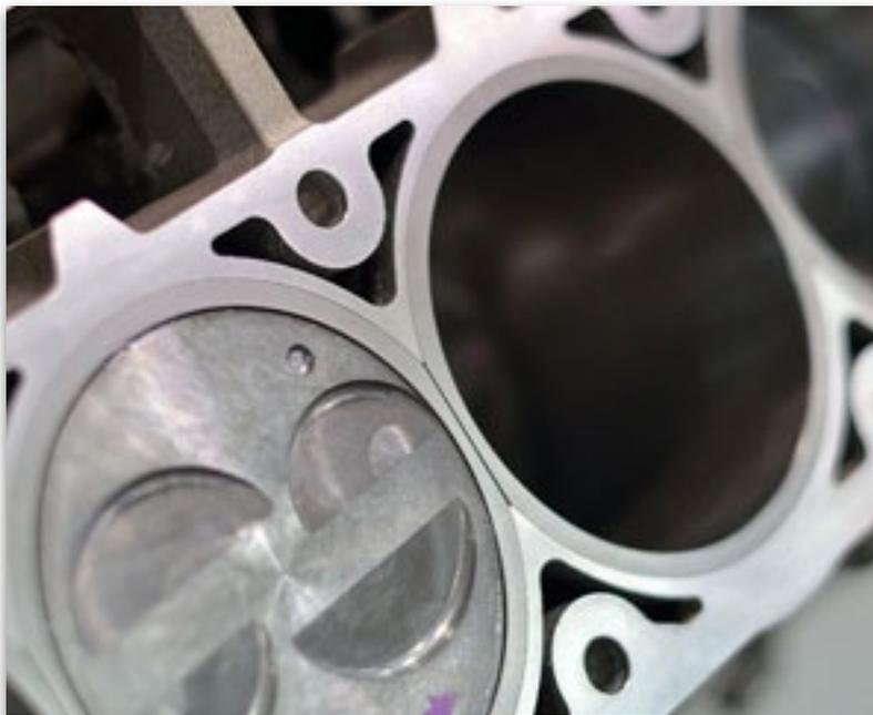
*The pressed-in liners are siamesed for about a two inch section where two liners would interfere. There's no decrease in wall strength because the flat surfaces of the two liners support each other. Image: GM Powertrain.*
