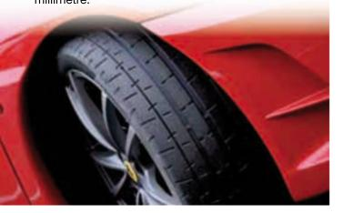
In front (for cars with different sections on the axles) and allaround fitments, the longitudinal grooves in this zone have greater width - to counter the effects of standing water - with respect to the rear tyre.
