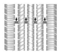
Treadwear indicators are one way to tell when it is time for new tires. Treadwear indicators appear when the tires have only 1.6 mm (1/16 in) or less of tread remaining. See *Tire Inspection on page 10-72* and *Tire Rotation on page 10-72*.
