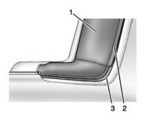
6. Push the edge (2) of the center of the tonneau cover (1) under the vehicle trim (3).
