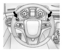
Vehicles with any axle other than GW8 have a Tap Shift Mode. Tap Shift allows you to manually control the automatic transmission. To use Tap Shift, the shift lever must be in M (Manual Mode). Vehicles with this feature have indicators on the steering wheel. The controls are on the back of the steering wheel. Tap the left control to downshift, and the right control to upshift. The DIC display indicates the gear the vehicle is in.
