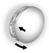
The fuel cap is behind a hinged fuel door on the passenger side of the vehicle. If equipped, the fuel door is locked when the vehicle doors are locked. Press on the RKE transmitter to unlock. To open the fuel door, push and release the rearward center edge of the door.
