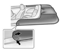
Grip the tonneau cover at the notch and pull back to release the tab on both sides.
