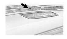
The vehicle has a light sensor on the top of the instrument panel. Do not cover this sensor or the system will come on whenever the ignition is on.
