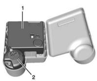
6. Remove the compressor (1) and the sealant canister (2).
