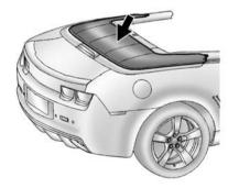
2. Unfold and place the tonneau cover on the vehicle.
