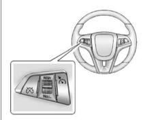
নৈ: Turns the cruise control system on and off. A white indicator light comes on in the instrument cluster when cruise control is on.
