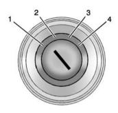
The ignition switch has four different positions.
