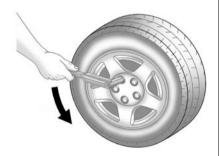
Use the fully extended wheel wrench to loosen all the wheel nuts one-half turn counterclockwise. Do not remove them yet.
