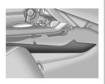
Pull the passenger side console trim away from the front half of the console to expose the shift lever mechanism.
