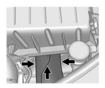
Press in on the tabs on the sides of the duct, and then push the duct rearward into the air cleaner/filter housing.
