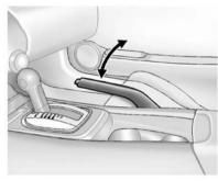
To apply the parking brake, pull up on the parking brake handle. It is not necessary to press the release button in while applying the parking brake. If the ignition is in the ON/RUN position, the brake system warning light will come on. See *Brake System Warning Light on page 5-19*.
