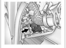
The instrument panel fuse block is on the end of the instrument panel, on the driver side of the vehicle. To access the fuses, open the fuse panel door by pulling out.
