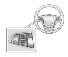
(On/Off): Turns the cruise control system on and off. A white indicator light comes on in the instrument cluster when cruise control is on.
