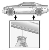
Position the jack lift head at the jack location nearest the flat tire. The location is indicated by a mark on the bottom edge of the vehicle. The jack must not be used in any other position.
