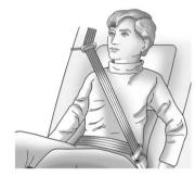
Buckle, position, and release the safety belt as described previously in this section. Make sure that the shoulder belt crosses the shoulder.
