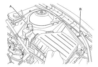
The jump start positive (A) and negative (B) posts are located in the engine compartment on the driver side of the vehicle.
