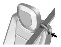
If the seat has a safety belt guide, and the safety belt is not routed through the guide, snap the guide around the belt webbing. Be sure the belt is not twisted.
