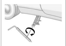
Raise the vehicle by turning the jack handle extension clockwise until the vehicle is far enough off the ground to allow enough room for the compact spare tire to fit under the vehicle.
