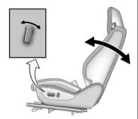
On vehicles with power reclining seatbacks the control is located on the outboard side of the seat.
