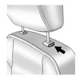
Pull the head restraint up to raise it. To lower the head restraint, press the button, located on the top of the seatback, and push the restraint down.
