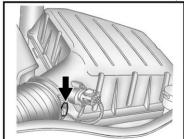
3.6 L V6 Engine Air Cleaner/Filter Housing shown (6.2 L V8 Engines similar)
