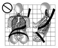
A: The shoulder belt is worn under the arm. It should be worn over the shoulder at all times.
