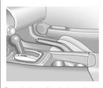
To apply the parking brake, pull up on the parking brake handle. It is not necessary to push in on the release button while applying the parking brake. If the ignition is in the ON/RUN position, the brake system warning light will come on. See *Brake System Warning Light on page 4-23*.
