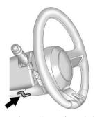
The lever is on the outboard side of the steering column.
