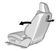
To access the rear seats pull up on the latch, located on the rear of the driver or front passenger seatback. Fold the seatback forward.
