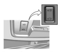
The sunroof can be opened without holding the switch down. Push the switch in the open direction until the second pause. The sunroof will fully open.
