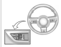
The cruise control buttons are located on the outboard side of the steering wheel.
