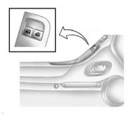
The power window switches located on the driver door control all windows. The window switches on the passenger door are only for that window. Push the front of the switch down to open the window. Pull the switch up to close it.
