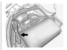
The electrical cord is located on the passenger side of the engine compartment, in front of the underhood fuse block for V6 models.
