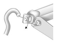
Fit the jack handle extension onto the jack by sliding the hook through the end of the jack.
