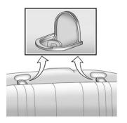
The top tether anchors are located on the rear seatback filler panel. Be sure to use an anchor located on the same side of the vehicle as the seating position where the child restraint will be placed.
