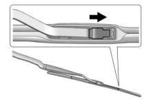
Lift up on the latch in the middle of the wiper blade where the wiper arm attaches.
