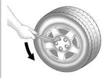
Use the fully extended wheel wrench to loosen all the wheel nuts one-half turn counterclockwise. Do not remove them.
