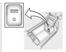
The AUX input is located in the center console.
