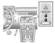
The power door lock switch is on the center console.
