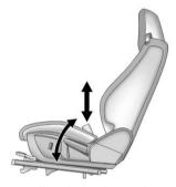
To manually raise or lower the seat, move the lever repeatedly upward or downward.
