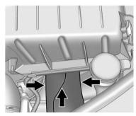
Press in on the tabs located on the sides of the duct and then push the duct rearward into the air cleaner/filter housing.
