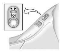
Vehicles with outside power mirrors have controls located on the driver door armrest.
