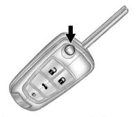
Press the button on the RKE transmitter to extend the key. Press the button and the key blade to retract the key.
