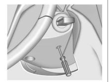
This vehicle is equipped with an electronic key lock release system. The key lock release is designed to prevent ignition key removal unless the shift lever is in P (Park).
