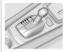
**P (Park):** This position locks the rear wheels. It is the best position to use when starting the engine because the vehicle cannot move easily.
