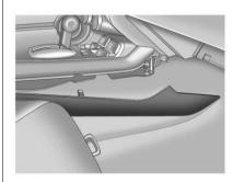
Pull the passenger side console trim away from the front half of the console to expose the shifter mechanism.
