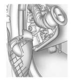
The instrument panel fuse block is located on the end of the instrument panel, on the driver side of the vehicle. To access the fuses, open the fuse panel door by pulling out.
