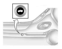
From inside the vehicle, press the button located on the driver door.
