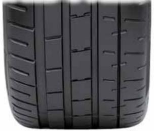
The asymmetrical tread pattern has two wide central ribs and large regular blocks. The inner area has greater groove density, whereas the outer area is derived from asphalt rally technology.
