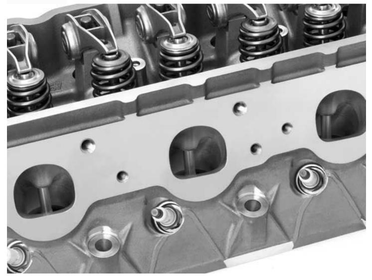
The deep CNC-ported exhaust ports are said to deliver 214 cfm of airflow at 28-inch water depression. Also visible are the beehive-shaped valves springs, which reduce critical mass and are less prone to harmonic disturbance than conventional parallel-wound springs. The small-diameter retainers also reduce mass at the valve side of the system.
