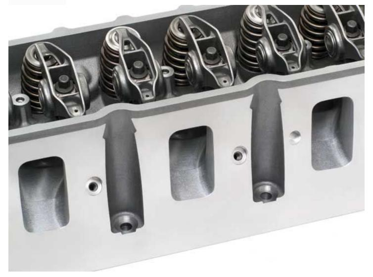
The intake ports are said to flow in the 360-cfm range at 28-inch water depression, and are fully CNC-ported. Ports feature a revised raised entrance and a larger cross section to work with the larger displacement of the LS7.
