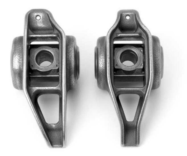
This paring of an intake and exhaust rocker illustrates the 9mm offset employed on the intake rocker (left). The offset alters the pushrod position outward, providing increased port width in an area normally constricted. The lightweight rockers are highly refined for low mass and inertia, and feature needle-bearing pivots. The rocker ratio has been increased to 1.8:1, amplifying the motions directed by the camshaft.
