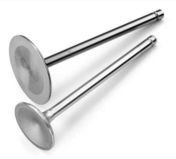
The intake and exhaust values are longer than the previous Gen IV values, providing room for deeper ports in the bowl area and over the port's critical short-side turn. The intake value is titanium, while the exhaust features a hollow sodium-filled stem for enhanced heat transfer.
