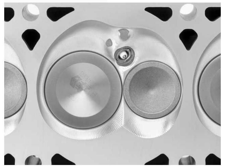
Combustion chambers are likewise fully machined to this masterfully sculpted form and are stuffed with enormous 2.200-inch intake valves and 1.61-inch exhaust valves. The valve angle in the cylinder heads relative to the decks has been altered to 12 degrees for enhanced airflow, a departure from the 15-degree angle employed by other Gen IV small-blocks. The chamber design offers significant quench area for efficient combustion.
