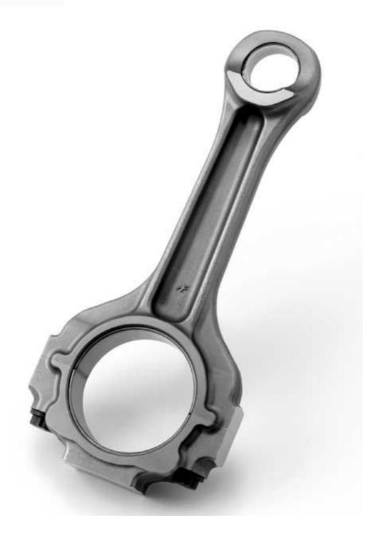
Titanium is used as the connecting-rod material, an exotic find even in racing engines. Strength, light weight, and fatigue resistance make it a worthy upgrade in a large, high-rpm engine like the LS7.
